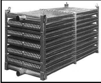
The coils are made of steel and welded to the collectors. The whole module galvanized after fabrication, as well as the support structure. The coils are equipped with spacing systems and supported by a galvanized steel structure. For specific cases, the modules can be manufactured in stainless steel.
