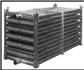
The coils are made of steel and welded to the collectors. The whole module is galvanized after fabrication, as well as the support structure. The coils are equipped with spacing systems and supported by a galvanized steel structure. For specific cases, the modules can be manufactured in stainless steel.
