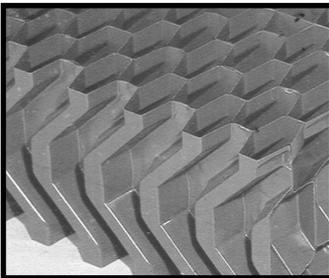
The drift eliminators are manufactured with PVC sheets with three changes of direction and drift losses lower than 0,002% of the design flow rate.
