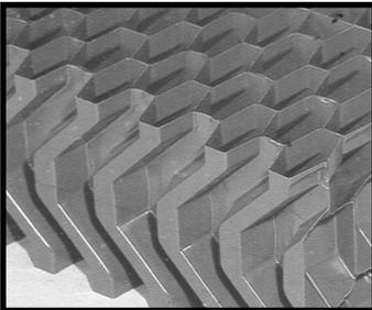
The drift eliminators are manufactured with PVC sheets with three changes of direction and drift losses lower than 0,002% of the design flow rate.
